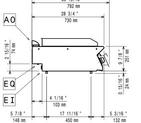
EI = Electrical inlet (power) EQ = Equipotential screw
